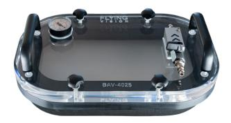
The BAV4025 is an NDT vacuum box designed for flat surfaces, tailored for leak testing welds, sheets, waterproofing membranes, and coverings on roof terraces, flat roofs in various industrial sectors. Its interchangeable base offers great flexibility to inspect different surfaces and weld configurations, enabling rapid leak detection.
