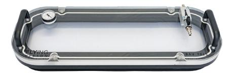
The BAV7025 is an NDT vacuum box designed for flat surfaces, tailored for leak testing welds, sheets, waterproofing membranes, and coverings on roof terraces, flat roofs in various industrial sectors. Its interchangeable base offers great flexibility to inspect different surfaces and weld configurations, enabling rapid leak detection.
